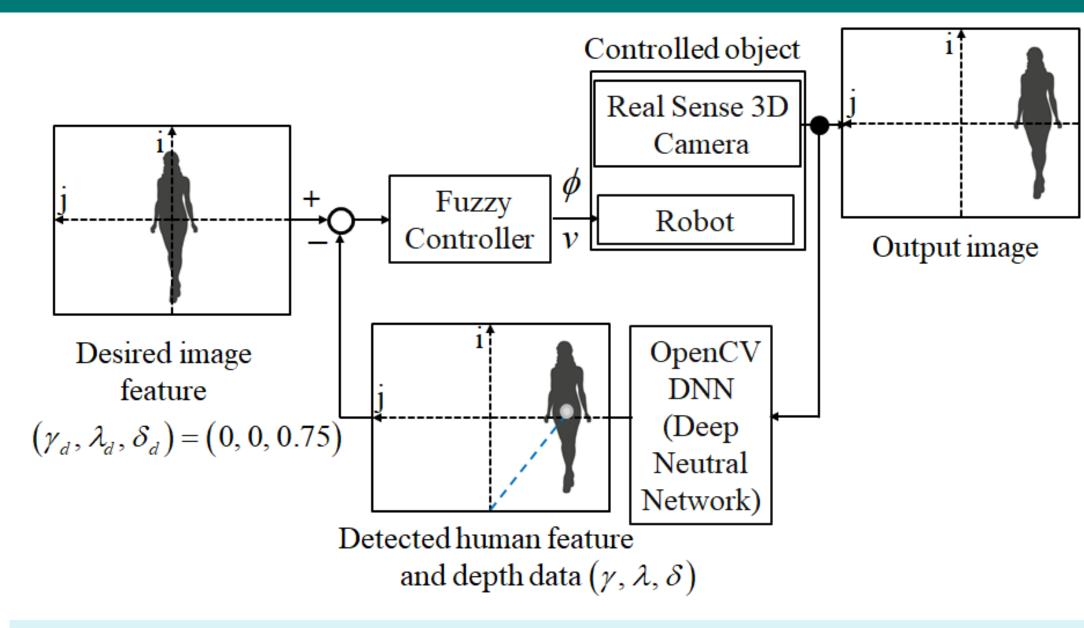
$\gamma, \lambda$  = the slope and intercept of the desired target line, v = the velocity of the robot,  $\phi$  = the steering angle of the robot, x, y,  $\theta$  = the position and orientation of the robot
